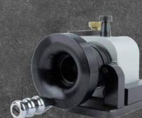
Countersink Sharpening Attachment\* LEX150INTL Standard: 1 flute Optional: 3 & 6 flute Max CS Diameter: 28mm
