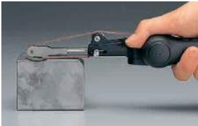
Grinding a flat surface
