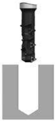
1. Positioning the milling cutter above core hole, check and adjust the length.
