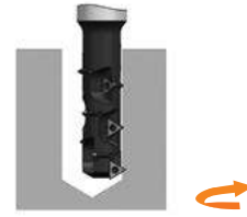
3. Circular interpolate cutting.
