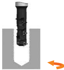
5. Circular interpolate cutting and retracting.
