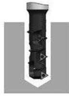
2. Get down to the request depth and check the radius.
