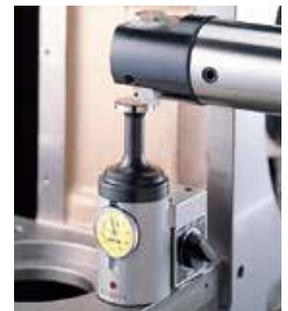
Also suitable for use of Micron Adjustment of Boring Arbor.
