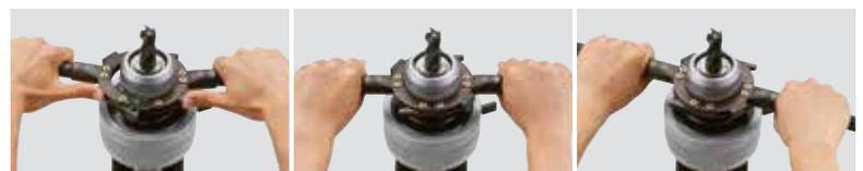
3 easy steps make it possible to clamp, unclamp milling chuck very safely and easily.
