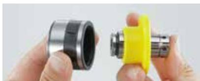
Collet removal (SKR-6) is supplied as standard only for SK6. SKR-10, SKR-16 and SKR-25 are available as an option. Collet removal is not necessary for the new types of collet (SK10 to SK25 collet including SK13 and SK20).
