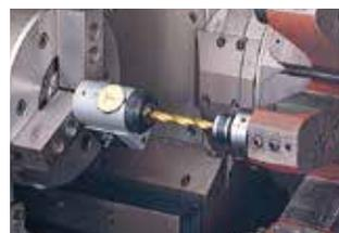
Example of usage at NC Lathe.
